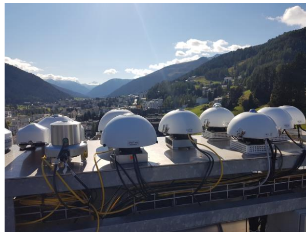
Pyrometers measuring longwave downward radiation
