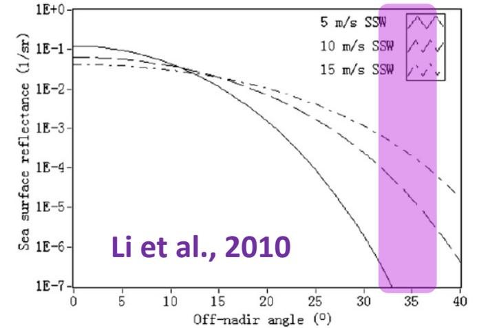
FIG. 4. Sea surface specular reflectance for different off-nadir angles and SSW at 355 nm.
