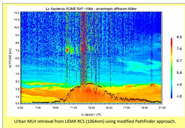
Urban MLH retrieval from LIDAR RCS (1064nm) using modified Pathfinder approach.
