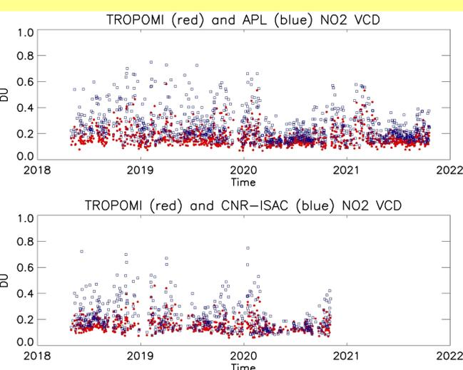
TROPOMI (red) and BAQUININ-PGN (blue) collocated NO<sub>2</sub> Total Column time series. Upper panel: APL (urban); lower panel: CNR-ISAC (semi-rural). For matchup data and methodology see: <https://mpc-ndaf-server.tropomi.eu/>
