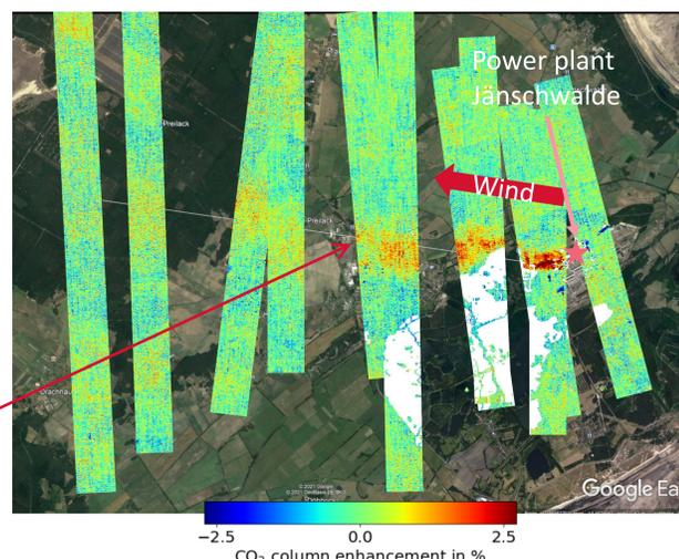
Measurement flight over coal fired power plant Jänschwalde. The non binned flight track sections orthogonal to the plume are overlayed over Google Earth imagery. The emission plume is visible up to 10 km away from the power plant; Background Image: Google Earth, [earth.google.com/web/](http://earth.google.com/web/)
