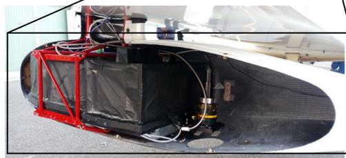
Sensors in the underwing pods may have a gross weight of up to 45 kg on each side of the aircraft. Electrical power is provided by a 28 VDC/50 A bus system.
