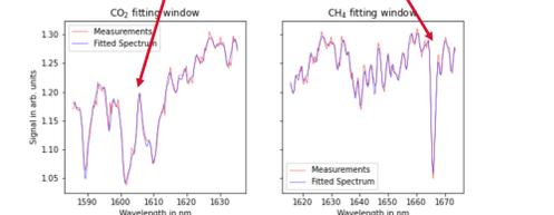
Retrieval of CH<sub>4</sub> and CO<sub>2</sub> enhancements out of the acquired spectra in two fit windows using the WFM-DOAS retrieval (Krings et al., 2011) results in column scaling factors for CH<sub>4</sub> and CO<sub>2</sub>
