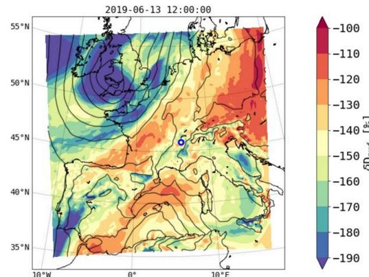
Figure 3:  $\delta D_{pwrf}$  (colors) and sea level pressure (black contours) in COSMO<sub>ISO</sub> at 12 UTC 13 June 2019. The blue circle denote the location of Anney.
