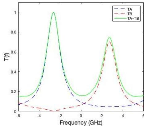
Rayleigh channel (FPA and FPB) transmission curve
