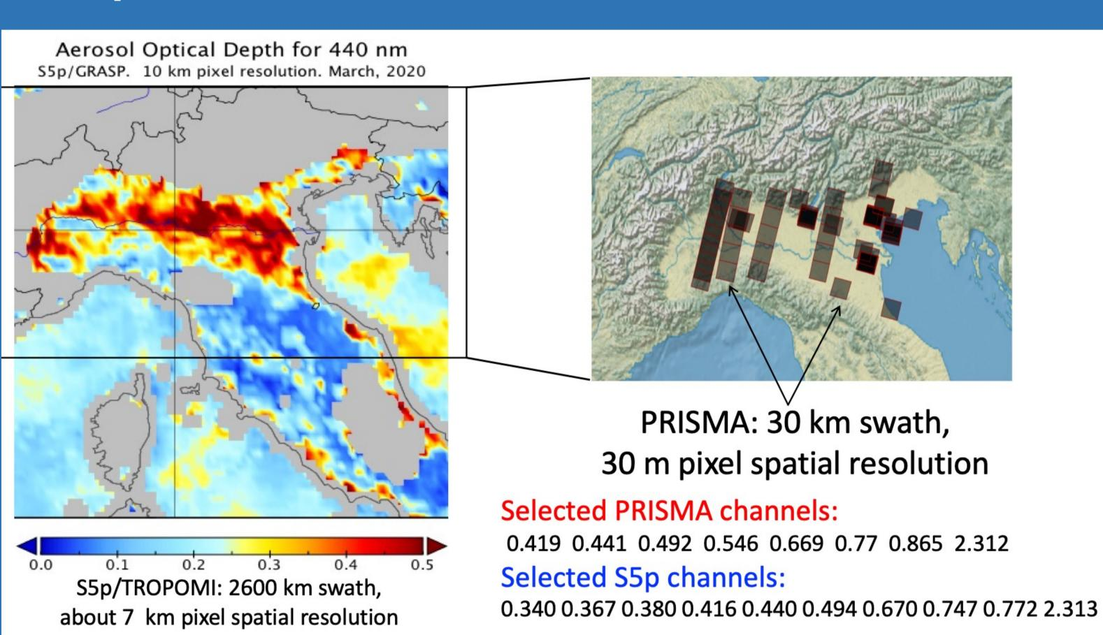
S5P/TROPOMI provides global hyperspectral measurements in wide spectral range which can be beneficial for aerosol and surface characterization
